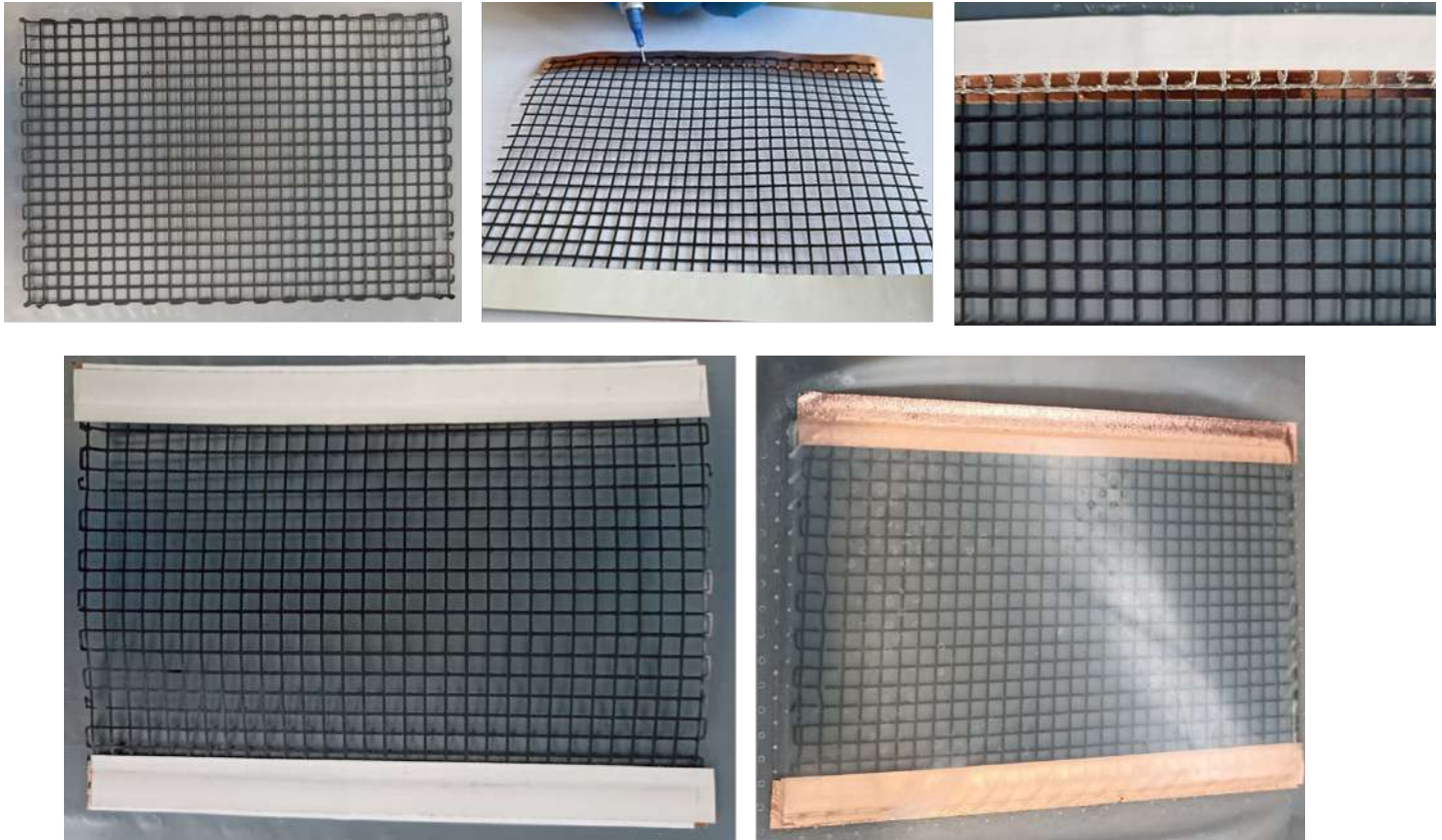
Figure 53 CNT-based grid – connection preparation and GRFP element with embedded heater
