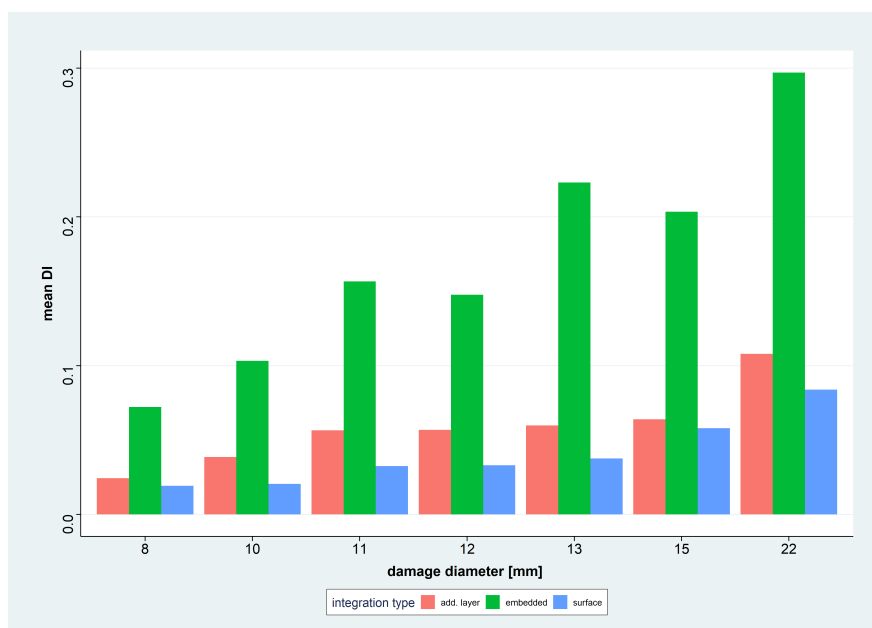
Figure 44: Comparison of PZT sensors sensitivity to artificial damage after cyclic loading test with respect to different techniques of sensors integration with the composite structure
