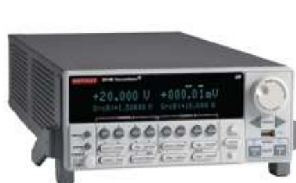
Figure 15. Measuring source Keithley 2614B and operational parameters of the Keysight E4980A LCR meter.
