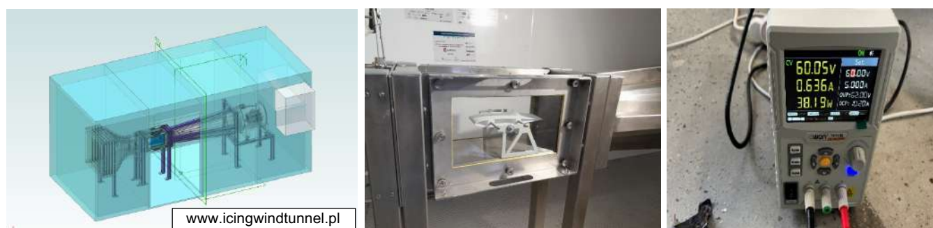
Figure 56: Icing wind tunnel set up and tests parameters of power supply
