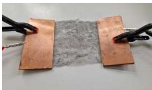
Figure 16. Metallized PPS veils connected with measurement system
