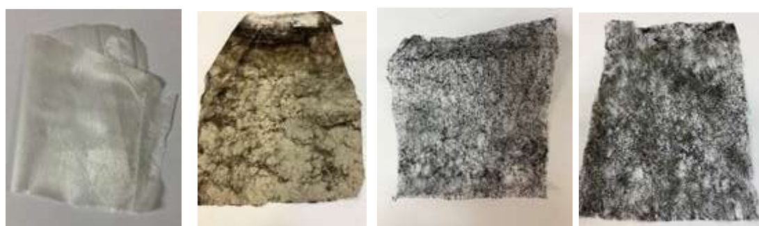
Figure 10. From the left: neat coPA veil before metalization; coPA veil after metallization; PPS veil with 1wt% CNT before metallization; PPS veil with 1wt% CNT after metallization.
