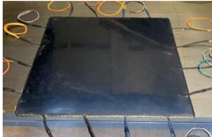
Figure 36 Specimen with embedded PZT sensors after curing
